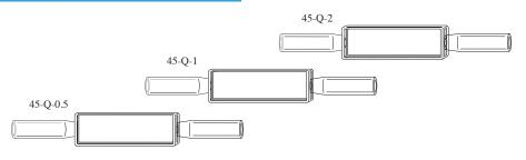
The inlet/outlet tube dimensions are 25mm long: Up to 2mm pathlength: 2mm ID, 4mm OD 5mm pathlength: 5mm ID, 7mm OD
